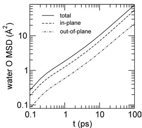
**Fig. 3** Mean-squared displacements (MSD) computed from molecular dynamics trajectories of oxygen atoms of hydration water molecules between purple membrane stacks at 296 K. Solid: total MSD (three-dimensional). Dashed: components of the MSD in the plane of the membranes (two-dimensional). Dot-dashed: component of the MSD normal to the plane of the membranes.
